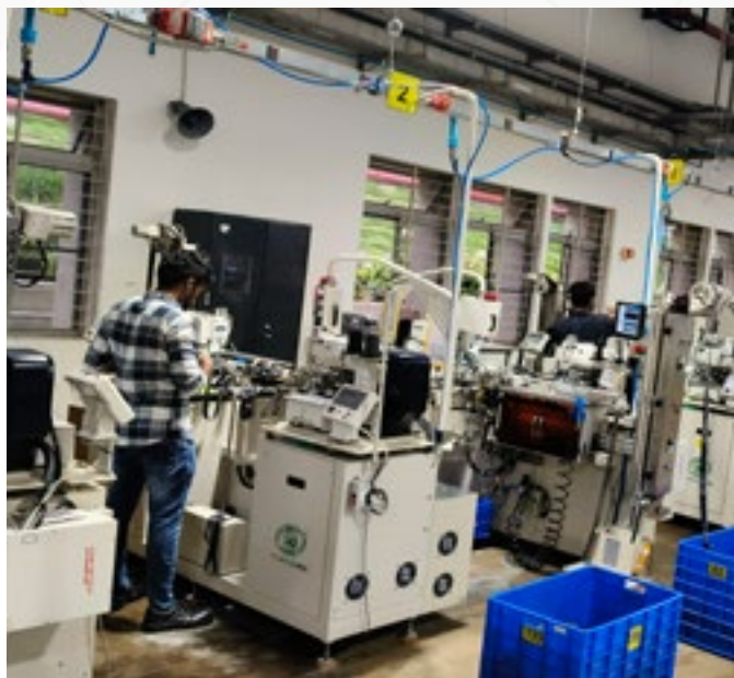
Automated elastic ring making machine
